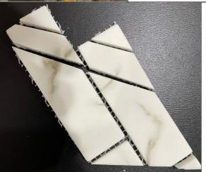
Cutting the RG 1x4 Herringbone on a 45 can be a problem, as the small tips tend to break.
